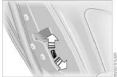
With through-loading system: tilt the backrest halfway forward to make the cover easier to remove, refer to page 106.
